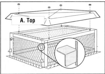
2. Bend the inserted tabs (as illustrated) by hand. Bend tabs in opposing directions on each corner for strongest construction. Complete the base assembly by completing this procedure on each corner. Place Top (A) over the assembled base and secure the Top to the base with the four 5/16" Nuts (D).
