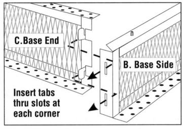
1. Place a Base Side (B) on a flat working surface with the solid flange and welded bolts facing upward and the perforated flange facing downward and to the outside. Place a Base End (C) perpendicular to the Base Side with the top flange facing inward and the bottom flange facing outward. Insert the two (2) tabs on the Base End through the slots on the Base Side.
