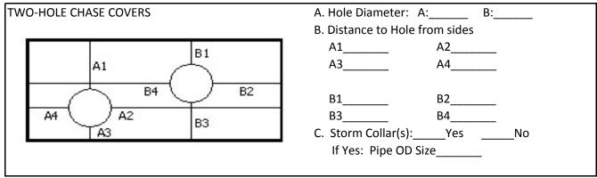
HY-C will add up to 1/4" to reported Perimeter Dimensions to ensure fit/clearance. Hole Diameters will be made 1/2" larger than reported to ensure fit/clearance.
